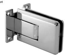
This innovative Atlas Series Hinge gives you the best of two worlds. It combines minimal hardware and is all wrapped up in this stylish, heavy-duty Hinge. Two of these double-acting Hinges will allow you to create 'all-glass' doors weighing up to 140 pounds (64 kg) with a maximum width of 39" (1 m). **NOTE:** Do not exceed two Hinges per door.
