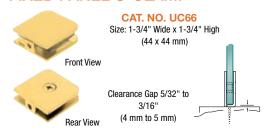
Fixed Panel U-Clamps mount directly to the wall, ceiling or floor to secure vertical fixed glass panels. Clearance between the glass and wall is from 5/32" to 3/16" (4 mm to 5 mm). RTV408C Clear Silicone can be used to provide a waterproof seal.
