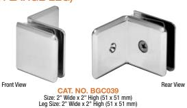
Clamps mount directly to the wall, ceiling or floor to secure vertical fixed glass panels. Clearance between the glass and wall is 1/16" (2 mm). RTV408C Clear Silicone can be used to provide a waterproof seal. 90° leg provides extra strength. Larger mounting leg covers more tile area.
