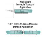
Movable Transom Clamps can be used to pivot transom panels above the shower door. Wall Mount and 180° Glass-to-Glass Clamps can be used in combination, depending upon the configuration of the enclosure. Replacement Nylon Washer is Cat. No. 90295A120.
