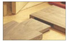
We incorporate the best wood working techniques on the market - mortise and tenon construction. It is a proven way of construction that won't sag or fail over time.
