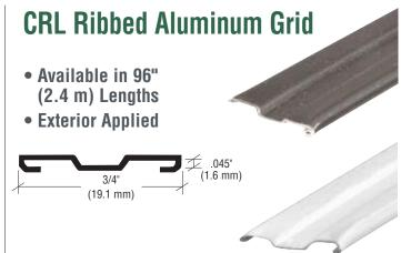
This CRL Ribbed Aluminum Grid stock is designed to be installed onto existing glass windows to produce a French or Colonial window appearance. The Grid is applied to the window surface using Cat. No. RTV408C Clear Silicone as an adhesive.
