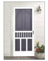
CRL Hinged Vinyl Screen Doors do not require cutting, never need painting, and will not peel, chip or splinter. Clean with soap and water for easy maintenance. They feature a separate hinged-bar for easy handing choices. The bottom expanders allow for a perfect fit every time. The door frame is 3" (76 mm) wide x 7/8" (22 mm) thick.
