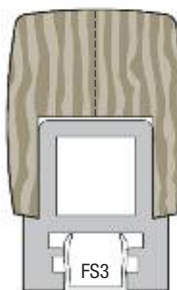
597 Series 1-3/4" x 2-3/4" (45 mm x 70 mm) Hand Rail Shown With Optional FS3 Snap-In Pocket Filler
