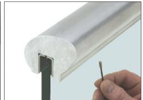
NOTE: Each Cap Rail comes complete with pre-drilled holes 24" (610 mm) on center and set screws along one side of the Cap Rail for proper attachment to the Adapter Strips.
