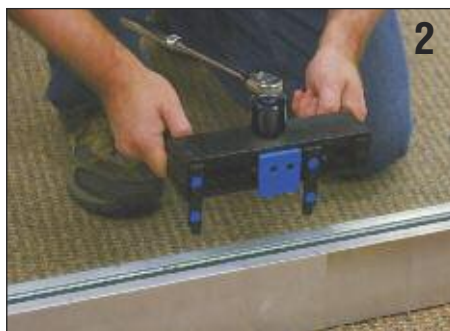
Place the TAPER-LOC® Installation/Removal Tool into position directly over the Taper Set.
