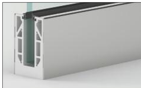
Install the Glass Panel and insert, then tighten the TAPER-LOC® Tapers with the TLK12 Tool to lock the glass securely in place. Roll-in the Inside Safety Seal and you're done.
