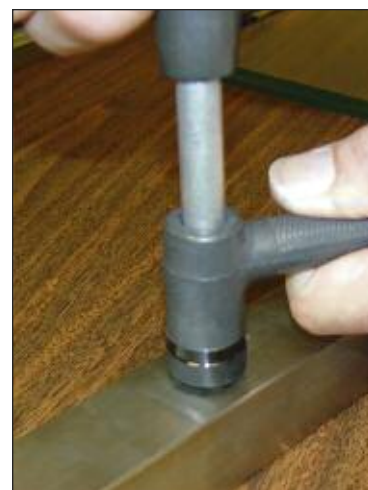
Riv-Nut Steel Insert Fastener installed in Square Tubing
