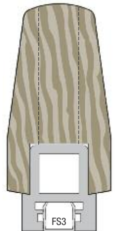
572 Series 2" x 4-1/2" (51 mm x 114 mm) Hand Rail Shown With Optional FS3 Snap-In Pocket Filler
