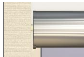
4. Secure Cap Rail to glass using 95CBL Silicone and Shims.
