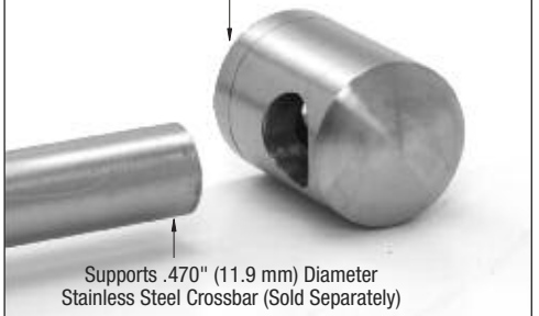
7/8" (22 mm) Diameter Standoff Connector Supplied With Flat Back Adapter
