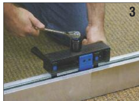
Tighten the TAPER-LOC® components using our measured Torque Wrench and you are done.
