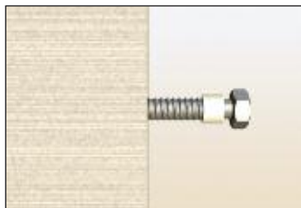
2. Install Lag Screw with Nylon Spacer at required location on the substrate.
