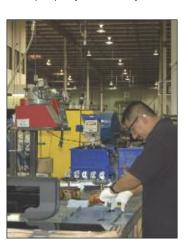
Fixtures and Welding - Precise and accurate fixtures guarantee constant and repetitive results. Having all component parts securely fastened prevents warping and mis-alignment during the welding process.
