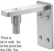
This CRL Wall Mount Gate Pivot is designed for mounting to a post or wall. As a safety measure the bottom of the pivot bar is raised 3/4" (19 mm) above the CRL Top Gate Patch Fitting (not included), allowing for adequate space to help prevent pinching of fingers. Available in brushed stainless steel finish, it comes complete with instructions and a glass cut-out template. Minimum order is one each.
