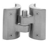
This CRL Tubing Hinge is designed to work with 1.9" (48.3 mm) diameter tubing. The Hinge is free-swinging, and pivots on a nylon bearing. Hinge is secured from the front side with supplied screws. Maximum width 42" (1067 mm); maximum weight 65 lbs. (29.5 kg). Minimum order is one each.
