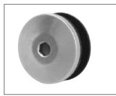
CRL Surface Mount Cap Assemblies work with eight different Column or Arch Swivel Fittings. Each Cap is supplied with all necessary gaskets. Fittings are tightened with a 6 mm Allen wrench (not supplied). Thread pitch is M18 x 1 mm. See below for glass fabrication requirements.
