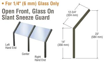
Our Open Front, Glass On Slant Sculptured Series Aluminum Sneeze Guards are in stock and ready for immediate shipment. The 1-5/16" (33.3 mm) Square Post is available in three styles and three finishes. Easily attaches to the counter. Ships knocked-down. Use Cat. No. 32629 Metal Contact Cement (see page P602) to achieve a secure and permanent bond at all connections.
