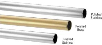
CRL Tray Slide Shelf Tubing is used to create a sliding tray shelf in front of a food service island. The 1" (25.4 mm) Tubing mounts with screws on the Tray Slide Shelf Brackets, spaced no more than 42" (1067 mm) apart.
