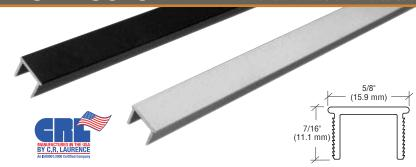
Post Pocket Fillers are designed to be snapped into the glass pocket of the Posts where glass will not be used. No tools or adhesives are required, and they can be removed to reconfigure post layouts if required. All Post Pocket Fillers are low maintenance, with a special coating to prevent corrosion. Fillers are available in the same seven standard colors as our Partition Posts, plus unfinished chromate. Custom colors are also available.
