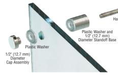
Install Hanger Bolt into stud or wall anchor. Then slip on the non-threaded Standoff Base, Plastic Washer, panel material, Plastic Washer, and attach the Cap.
