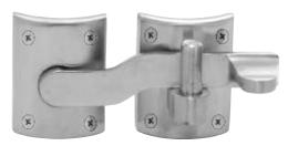
This CRL Tubing Latch is designed to work with 1.9" (48.3 mm) diameter tubing. Latch has a manually operated pivoting bar, and is secured from the front side with supplied screws. Minimum order is one each.
