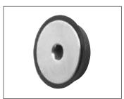
CRL Flush Mount Cap Assemblies work with eight different Column or Arch Swivel Fittings. Each Cap is supplied with all necessary gaskets. Fittings are tightened with a 6 mm Allen wrench (not supplied). Thread pitch is M18 x 1 mm. See below for glass fabrication requirements.
