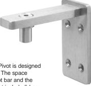
This CRL Wall Mount Door Pivot is designed for mounting to a post or wall. The space between the bottom of the pivot bar and the CRL Top Door Patch Fitting (not included) has been reduced to 1/8" (3 mm), because at gate height the chance of pinching fingers is greatly reduced. Available in brushed stainless steel finish, complete with instructions and a glass cut-out template. Minimum order is one each.
