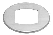
CRL's Garnish Rings add the finishing touch to your installation. These 316 Grade brushed and polished stainless steel covers easily slip over the Frameless Windscreen Clamp, and secure in place with Cat. No. 95CBL Black Silicone (see page P628).
