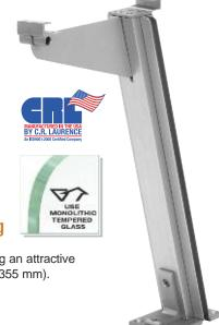
The D996 Design Series Slant Front Post angles forward at 74 degrees to the countertop, providing an attractive look that is popular for cafeteria use. It is available with Top Brackets in widths from 6" to 14" (152 to 355 mm). Intermediate Brackets are not available. The glass channel is full post height.
