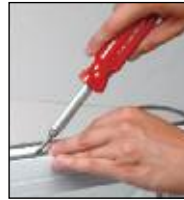
Press new pile into groove with screwdriver
