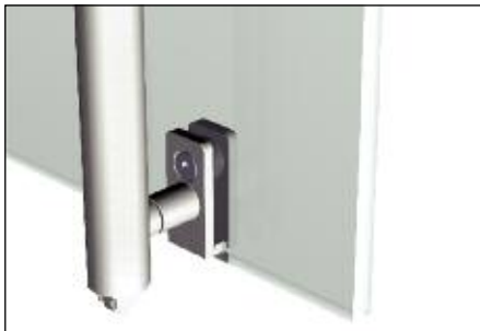
Glass Mount Detail at Latch
