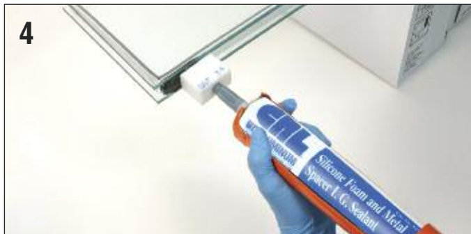
Apply CRL Hot Melt Butyl or Cat. No. 877 Sealant to seal the unit.
