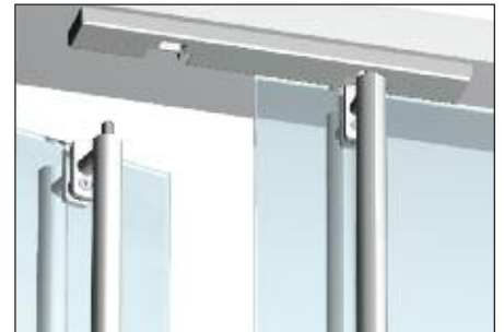
Glass Mount Detail at Latch With Header and ESK Strike
