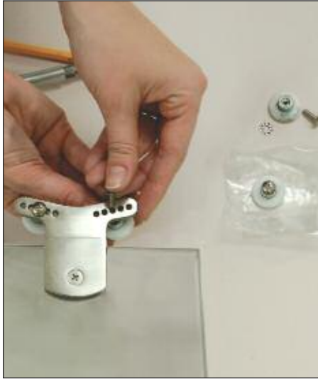
Replacing Damaged Rollers
