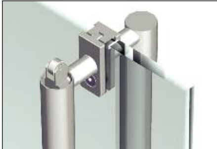
Glass Mount Detail at Latch
