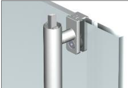
Glass Mount Detail at Latch
