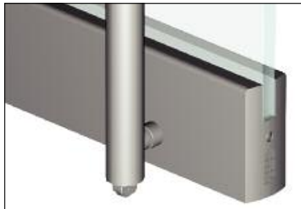
Rail Mount Detail at Latch
