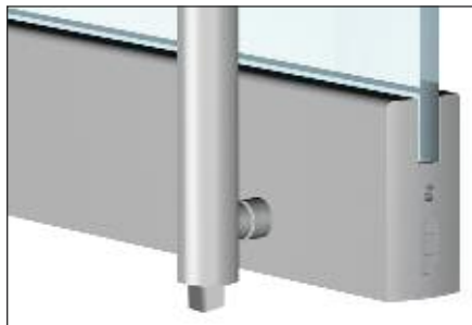
Rail Mount Detail at Latch
