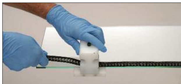
Apply Duralite® to clean glass surface with Applicator or by hand.
