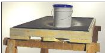
67 pound bucket placed on the screen panel for 21 days, then removed.
