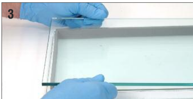
Index second piece of clean glass and press on to Super Spacer®.
