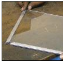
Install miter cut frame with adhesive onto glass
