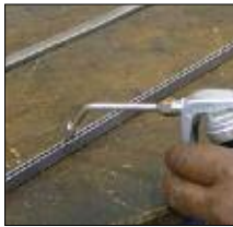
Using C205GL Adhesive and 195AG Pump, dispense adhesive into frame
