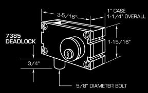
THIS BLUMCRAFT DEADLOCK HAS A 5/8" DIAMETER DROP BOLT WITH A 3/4" THROW THAT CAN ENGAGE INTO A STRIKE PLATE, THRESHOLD, OR DUST-PROOF STRIKE. THE 7385 LOCK CAN BE MOUNTED IN THE BLUMCRAFT 64OC DOOR AND MOST TEMPERED GLASS DOORS. STANDARD MORTISE KEY CYLINDERS ARE HELD IN POSITION WITH SET SCREWS THAT ARE ACCESSIBLE FROM THE END OF THE DOOR RAIL.
