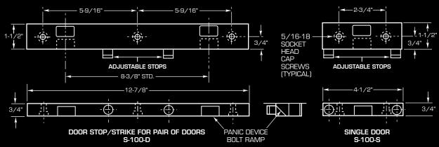
NOTE: DOORSTOP/STRIKES FOR DEADBOLT HOUSINGS ARE SIMILAR TO THE ABOVE, EXCEPT THAT THEY HAVE NO PANIC BOLT RAMP. MOUNTING HOLES ARE IDENTICAL.
