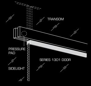
THE TRANSOM BAR IS HELD IN PLACE USING PRESSURE PADS AT THE SIDELIGHT AND SUPPORT RODS HANGING FROM THE CEILING CHANNEL
