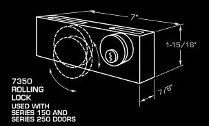
THIS BLUMCRAFT DEADLOCK HAS A CYLINDRICALLY SHAPED BOLT THAT ROLLS RATHER THAN SLIDES. ROLLING REDUCES THE CONTACT AREA SURROUNDING THE BOLT AND THE POSSIBILITY OF FREEZING IN AN OPEN OR CLOSED POSITION. WHEN LOCKED, THE BOLT BECOMES VERY DIFFICULT TO DAMAGE BECAUSE IT REVOLVES ON ITS OWN AXIS. BALL BEARINGS SMOOTH OUT THE OPERATION OF ALL STAINLESS STEEL MOVING PARTS. SIX PIN MORTISE CYLINDERS ARE STANDARD AND CAN BE KEYED ALIKE OR KEYED SEPARATELY.
