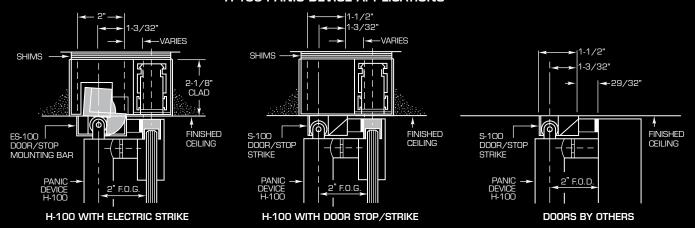
NOTE: SH-100 SWITCH HOUSINGS, WHILE SIMILAR IN APPEARANCE TO H-100 PANIC DEVICES, HAVE A SWITCHING FUNCTION THAT ONLY OPERATES INDEPENDENT ELECTRIC LOCKS. THESE ELECTRIC LOCKS CAN BE ELECTROMAGNETIC, DROP BOLTS, OR SHEAR LOCKS. CONTACT BLUMCRAFT WITH MODEL NUMBER OF SELECTED LOCK TO INSURE COMPATIBILTY.
