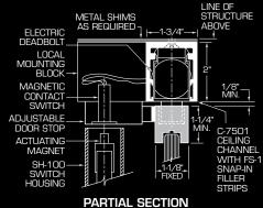
NOTE: RAILS CAN BE ADAPTED FOR VARIOUS TYPES OF ELECTROMAGNETIC LOCKS OR ELECTRIC DEADBOLTS, CONTACT BLUMCRAFT WITH MODEL NUMBER OF SELECTED LOCK TO INSURE COMPATIBILITY.
