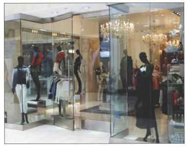
CRL 10" (254 mm) Square Shape Full Length Door Rails have been designed to meet requirements mandated under the 1998 Amendments to the ANSI A117.1 Guidelines and Standards for accessibility to buildings and facilities of people with disabilities. This section provides a 10" (254 mm) surface from the floor across the bottom of the door.
