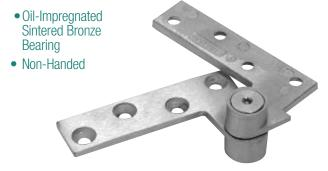
These Offset Top Pivots are supplied with an oil-impregnated sintered bronze bearing, and intended for use with standard aluminum, wood, and hollow metal doors. These Pivots are fully mortised and non-handed. They are supplied with wood and machine screws to allow most common installations.
