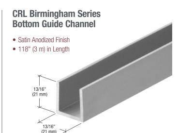
The CRL Birmingham Series Bottom Guide Channel is recessed into the floor, and receives the guide pin from Cat. No. B1R19 and B1R21 to secure and guide the panels of the bi-fold systems. This Channel is made from satin anodized aluminum and is 118" (3 m) in length.
