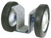
With the CRL Two-Wheel Adjustable Glass Dolly, heavy items such as railing panels, storefront doors, framed windows, storm windows, I.G. units or just about any other flat surfaced item can be easily moved in an upright position. The Dolly is adjustable to widths from 2-1/2" to 4-1/2" (63 to 114 mm). The steel carriage is carpeted to prevent marring of the surfaces. Minimum order is one each.
