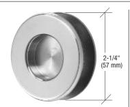
The CRL Thru-Glass Pull Handle has a recessed low profile design that screws together to install. Its solid stainless steel construction makes this a rugged yet elegant solution for a pull handle for a sliding glass door. The thickness of this Thru-Glass Pull doesn't impede movement in front of wall or glass sidelites as it allows for full door opening access. It is supplied
