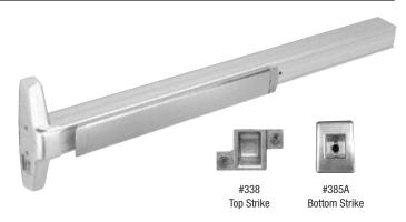
The Top Rod is adjustable from 80" (2032 mm) to 100" (2540 mm). Bottom Rod is adjustable from 35-5/8" (905 mm) to 49-5/8" (1260 mm). Extension Rod Kits for doors taller than 100" (2540 mm) are available on special order.
