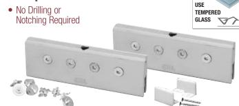
CRL EZ-Slide 80 Series Clamps and Bottom Guide are easily converted for use with 5/16" or 3/8" (8 or 10 mm) tempered glass. A pair of Clamps is rated for panels that weigh up to 176 pounds (80 kg). They grip the glass with precision-controlled pressure. No drilling or notching of the glass is required. Each pack contains two Clamps, Screws, and one nylon Bottom Guide.
