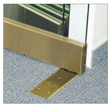
These CRL8300 Series Shallow Depth Floor Mounted Door Closers are preferred for many types of installations because they only require a shallow 1-9/16" (40 mm) cut-out in the floor. This is especially important on floors above the ground floor. The shallow cut-out leaves enough remaining floor under the Door Closer to support the door weight. The Door Closer has separate valves to control closing and latching speeds. Both 90 degree and 105 degree Hold Open and No Hold Open models are available.
