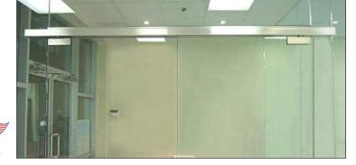
These Floating Headers for Overhead Concealed Door Closers allow the mounting of single or double doors off glass sidelites, with a transom above. Stock Floating Headers are for use in 1/2" (12 mm) glass-to-glass installations, and are prepared to accept CRL Overhead Concealed Door Closers and a 1/2" (12 mm) thick glass transom.
