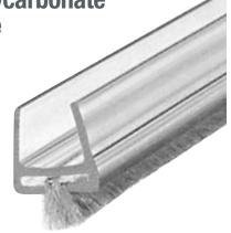
This CRL Clear Polycarbonate with Pile Weatherstrip prevents drafts from entering between glass doors. Simply snap over the edge of 1/2" (12 mm) glass. No tools required to install. Recommended clearance is 5/16" to 3/8" (8 to 10 mm). Stock lengths measure 98" (2.49 m) and can be shipped U.P.S. For replacement wool pile order Cat. No. A11435C.
