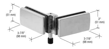
The CRL Birmingham Series Bottom Glass-to-Glass Guide Patch provides for smooth, simple bi-fold action where two panels meet in the bi-fold system. The guide pin works with the Cat. No. B1R17 Bottom Guide Channel, and mounts on the bottom corners of the glass panels. This Patch comes in a brushed stainless steel finish. Handing is easily field reversible. Two holes in each glass panel are required.
