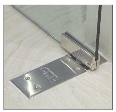
These CRL8400 Series Narrow Width Floor Mounted Door Closers are preferred on doors installed with Patch Hardware because smaller cover plates are more attractive in this type of installation. The Door Closer has separate valves to control closing and latching speeds. 90 Degree Hold Open and No Hold Open models are available.
