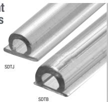
CRL Translucent Vinyl Bulb Seals can be used on inswing or outswing doors. SDTB closes gaps from 5/32" to 7/32" (4 to 5.6 mm); SDTJ closes gaps from 1/8" to 5/32" (3.2 to 4 mm). Available with or without pre-applied Very Hi-Bond Acrylic Tape. For additional information on Tapes, see below.
