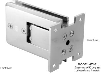
This innovative CRL Atlas Series 'All-Glass' Door Hinge gives you the best of two worlds; minimal hardware and self-centering action, all wrapped up in a stylish, heavy-duty Hinge. Two of these double-acting Hinges will allow you to create 'all-glass' doors weighing up to 140 pounds (63.5 kg) with a maximum width of 39" (1 m). NOTE: Do not exceed two Hinges per door.
