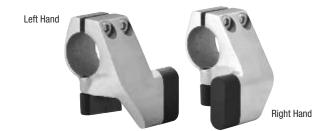
These Door Stops prevent 'over travel' of the door panels used in Laguna Series Assemblies with LS400 or LS500 Single Rollers, which helps protect the finished opening and the glass. Door Stops are installed by simply sliding them over the end of the Cat. No. LS104 Top Sliding Tube and then tightening them in place. NOTE: Left or right handing is determined as viewed from the hardware side of the opening.
