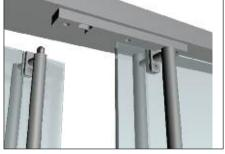
Glass Mount Detail at Latch With Header and PK Strike
