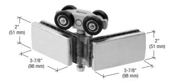
This CRL Birmingham Series Top Glass-to-Glass Roller Patch provides for smooth, simple bi-fold action where two panels meet in the bi-fold system. The double roller works with the Cat. No. B1R10 Top Track, and mounts on top corners of the glass panels. This Patch comes in a brushed stainless steel finish. Handing is easily field reversible. Two holes per panel in glass are required.
