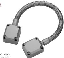
This CRL Armored Door Loop is designed to carry and protect the low voltage or monitoring cable between the door and frame. Standard finish is brushed stainless. 15-3/4" (400 mm) in length. Minimum order is one each.
