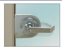
CRL's Lever Lock Glass Housings are easy to install and come complete with Housing and Lever Lockset for 3/8" or 1/2" (10 or 12 mm) thick glass. The Entrance, Storeroom, and Classroom models are available with either a Schlage® 'C' 6-Pin keyway or a 7-Pin Small Format Interchangeable Core (SFIC). See page 169Z for additional information. An ANSI 1-1/4" x 4-7/8" (32 x 124 mm) Strike is included.
