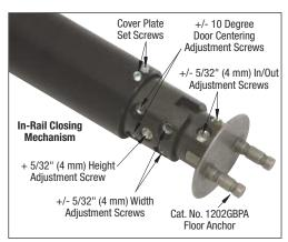
Bottom In-Rail Closing Mechanism with Floor Anchor
