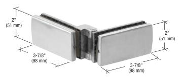
This CRL Birmingham Series Glass-to-Glass Patch connects two panels at non-roller locations in the bi-fold system. This Patch mounts on the top corners of the glass panels, and is also used at mid-height locations for openings taller than 104" (2.6 m). This Patch is available in a brushed stainless steel finish and is non-handed. Two holes in each glass panel are required.
