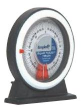
The CRL Magnetic POLYCAST® Protractor/Angle Finder measures any angle from 0 to 90 degrees in any quadrant. It comes with a dampened pendulum for quicker readings and an adjustable angle pointer for marking and transferring angles. The magnetic back and base provides "hands-free" use when working with ferrous surfaces. Minimum order is one each.
