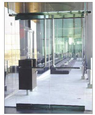
The CRL Blumcraft® B1250 Floating Transom System provides a clean, 'all-glass' look with minimal metal, and requires no holes or notches in the transom or sidelites. The Narrow Header of the B1250 is suspended from the C7500 Series Head Channel by thin stainless steel rods that are concealed in the gaps between the transom and sidelites.
