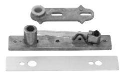
The CRL Jackson Center-Hung Pivot Set is designed to be used with standard 1-3/4" (45 mm) storefront aluminum doors weighing up to 250 pounds (113 kg). These Pivots fit top door rails with a depth of 1" (25 mm) and drops down 3/4" (19 mm) for full contact with the included Top Door Pivot Arm. Pin diameter is 1/2" (13 mm). These are perfect for new or retrofit applications.
