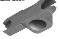
When used with a variety of Transom Patch Fittings, this Patch Keeper Insert allows the use of the AMR205 Lock on the top of the door. The Keeper Insert is put into the Transom Patch Fitting, and creates a receptacle for the lock's bolt.
