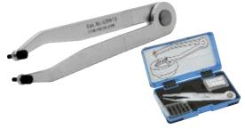
Use this CRL Universal Spanner Wrench as a quick and efficient method of attaching or loosening Spanners. Kit includes: one Adjustable Tool, five Metric (1.5, 2, 2.5, 3, and 4 mm) Spanner Pin Sets, five Fractional (1/16", 3/32", 1/8", 5/32", and 3/16") Spanner Pin Sets, and one Molded Carrying Case. The center-to-center distance between pins in the closed position is 1/4" (6 mm). Minimum order is one each.
