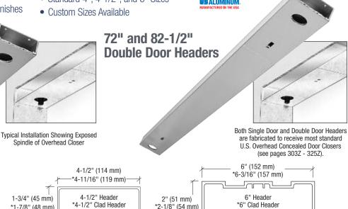
CRL Single Door Headers are fabricated to hold our overhead concealed door closers. Headers are carried in three stock sizes, and custom sizes can be special ordered. Headers are supplied with an Aluminum Mounting Clip for mounting the Header on the opposite side of the door closer. The door closer contains the mounting clip for that side of the Header. Snap-In cover plates allow for easy installation of the closer. **NOTE**: Clad and anodized Headers differ in size.
