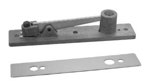
This Center-Hung Top Pivot fits top door rails with a depth of 1" (25 mm). Hardened steel pin has a diameter of 1/2" (13 mm), and drops down 3/4" (19 mm) for full contact with Top Door Pivot Arm.
