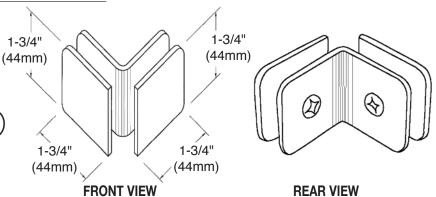
**Note:** The Clamps shown on this page can also be used in a wall-to-glass application. For information on this see pages 4X-7 and 4X-8.
