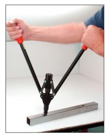
Third, compress the Rivet-Nut by using the CRL Cat. No. 34604 Heavy-Duty Thread Insert Tool (FIG. 2)
