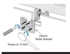
Place Glass Door on Wooden Shims to maintain 1/4" (6 mm) gap at bottom. Align notches in top of glass with Roller Brackets. Adjust height to fit.
