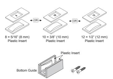
2. Use included screws to install on curb. Leave 9/16" (14 mm) gap between glass panels.
