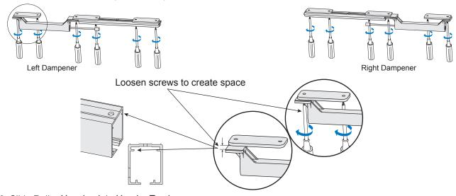
3. Slide Roller Housing into Header Track.
