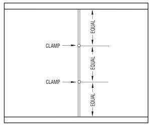
Two Clamps Equally Spaced
