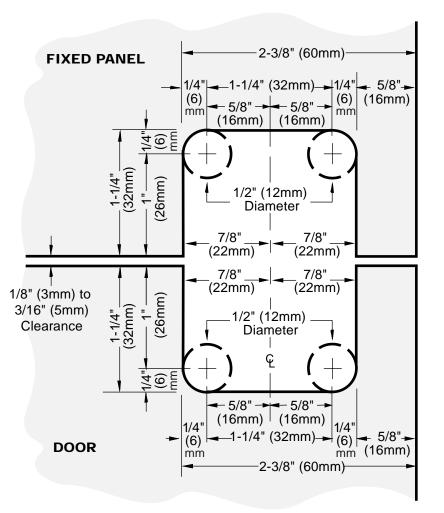
\* The 5/8" (16mm) measurement is ok as long as the fixed panel side clearance is the same as the door side clearance. If not, make the appropriate add-on or deduction.
