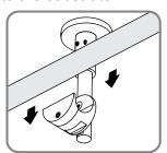
Loosen clamp to install sliding tube.
