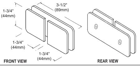
**Note:** The GCB182 and M0682 Clamp shown on this page can also be used in a wall-to-glass "Y" inline application. For information on this see pages 4X-23 and 4X-24.
