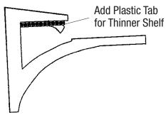
3. Install Shelf: Check thickness of shelf. Your Clips are either for 3/8" to 1/2" (10 to 12 mm) or 5/8" to 3/4" (16 to 19 mm). They are pre-set for the thicker capacity. If a thinner shelf is being used, peel mounting tape and carefully put Plastic Tab supplied in place (plastic side up-mounting tape down).
