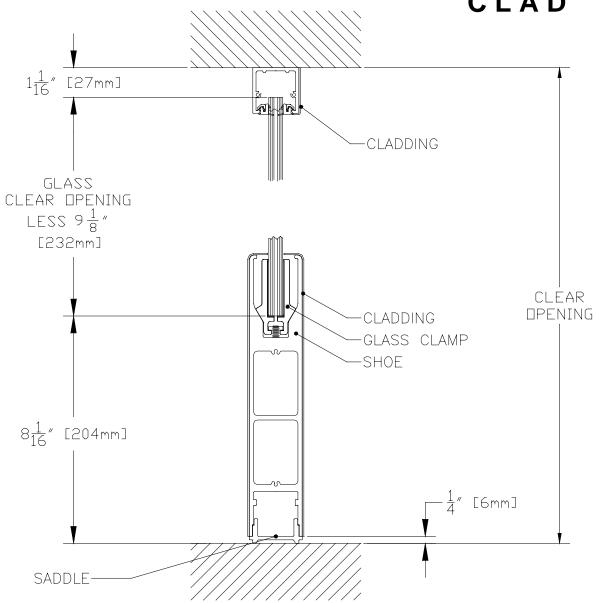
U-CHANNEL TOP CLAD OR NON CLAD 10" SQUARE SIDELITE RAIL CLAD ONLY WITH 1/4" SADDLE
