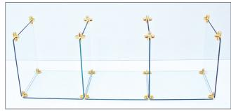
Step 2: Install the first row of vertical lites, this time attaching 3-Way Connectors at the top on the end lites and 4-Way Connectors at the top of the middle lites as shown in the illustration.
