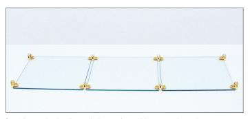
Step 1: Arrange the glass lites on the base surface which represent the number of cubes wide. Clean the bottom surface of the glass. As illustrated, attach 2-Way Connectors on the end lites and 3-Way Connectors between the lites. Use a wide blade screwdriver for Z-Line Connectors or a soft face rubber mallet for Clear Plastic Connectors.
