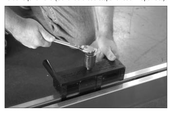
Make sure the blade movement mechanism of the TLK12 Tool moves freely, and hasn't become filled with dust or debris. Blade mechanisms that are poorly maintained may cause binding during the Taper compression operation, and result in an improper installation with insufficient compression of the Tapers.
