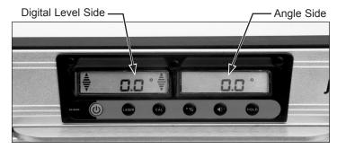
Display for Digital Level and Angle Locator.
