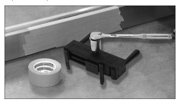
Step 3 Insert the Installation/Removal Tool into position, reverse the torque setting, and apply force to open the Tapers.
