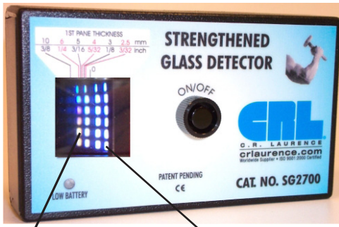
Figure 1: SG2700 inspecting a dual pane window. Note that one reflection column occurs for each glass surface.
