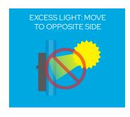
The Glass-Chek ELITE uses a laser to measure the thickness of the glass and air space. The unit may be affected by extremely bright lights or facing the sun directly. The screen will display this error message if this condition occurs. Simply move to a different location, go to the other side of the window, or shade the laser aperture. If the window is operable you may be able open the window and reach through the opening to block the incident light from the back side of the meter.
