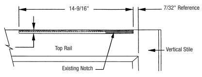
Mark Arm Clearance Slot as Shown Above. Rout Out Entire Clearance Slot on Interior Side Only.
